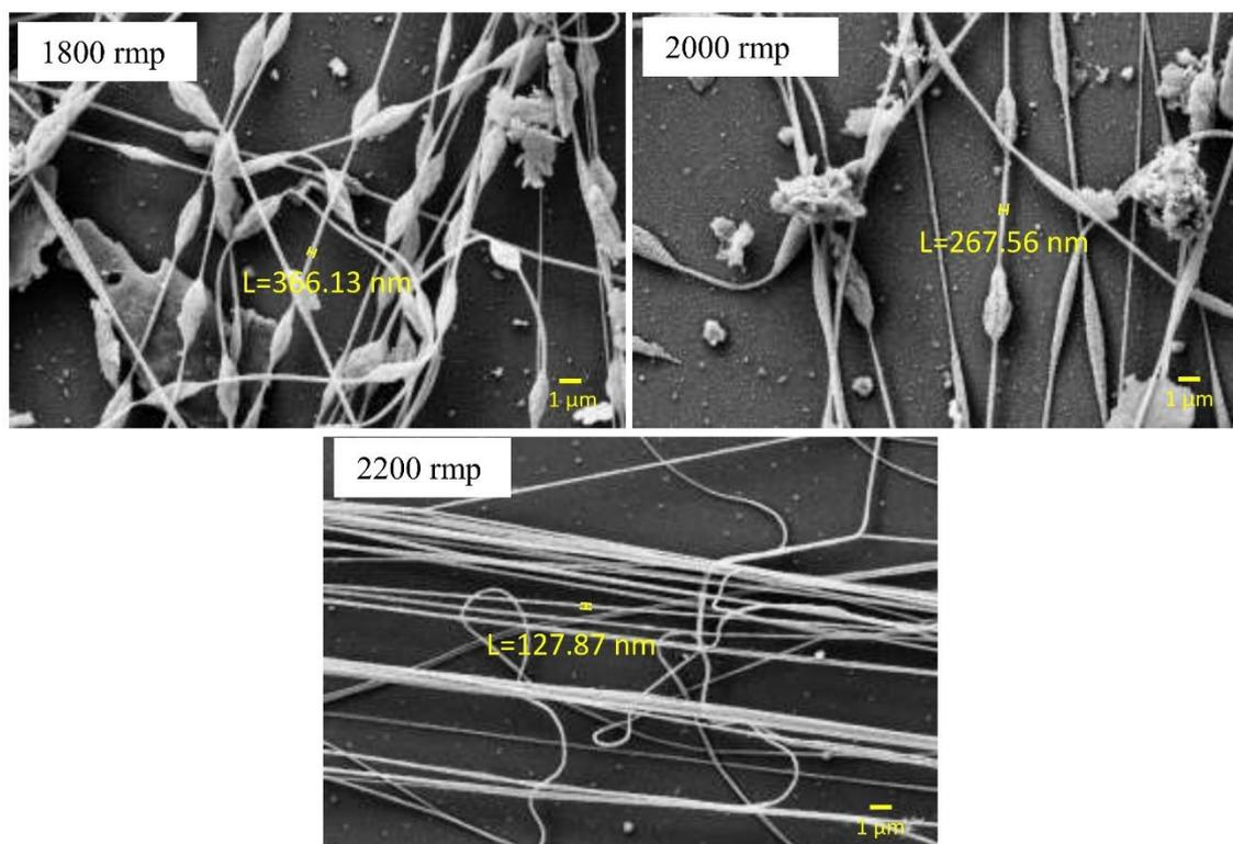
Fig. 1. FE-SEM images for the PMMA/TiO<sub>2</sub> nanofibers at different collector speed.
