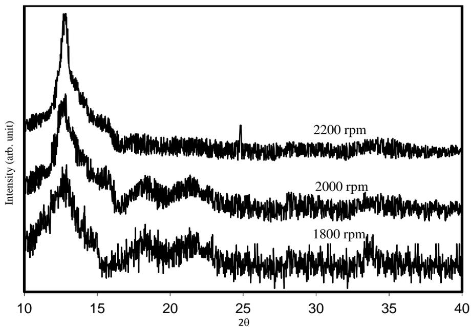
Fig. 2. The XRD spectra of the PMMA/TiO<sub>2</sub> nanofibers at different collector speeds.
