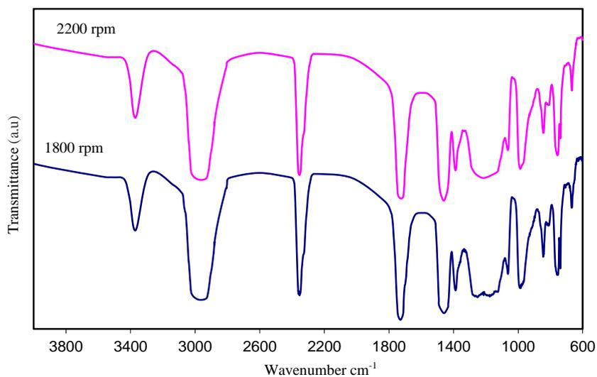
Fig.3. The FTIR spectra of of the PMMA/TiO<sub>2</sub> nanofibers at different collector speeds.
