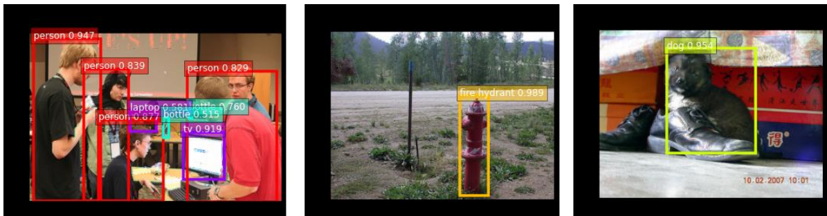
Figure 8. Sample of detection and classify objects based on proposed hybrid CNN_LSTM model
