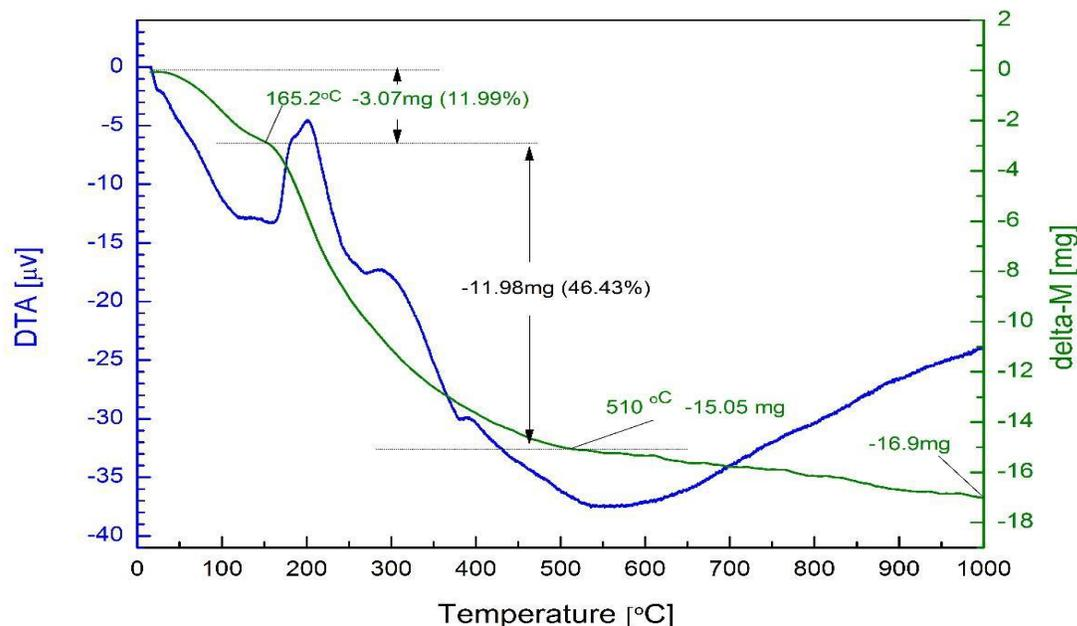
Fig(1) DTA and TGA The mass decreases with increasing temperature
