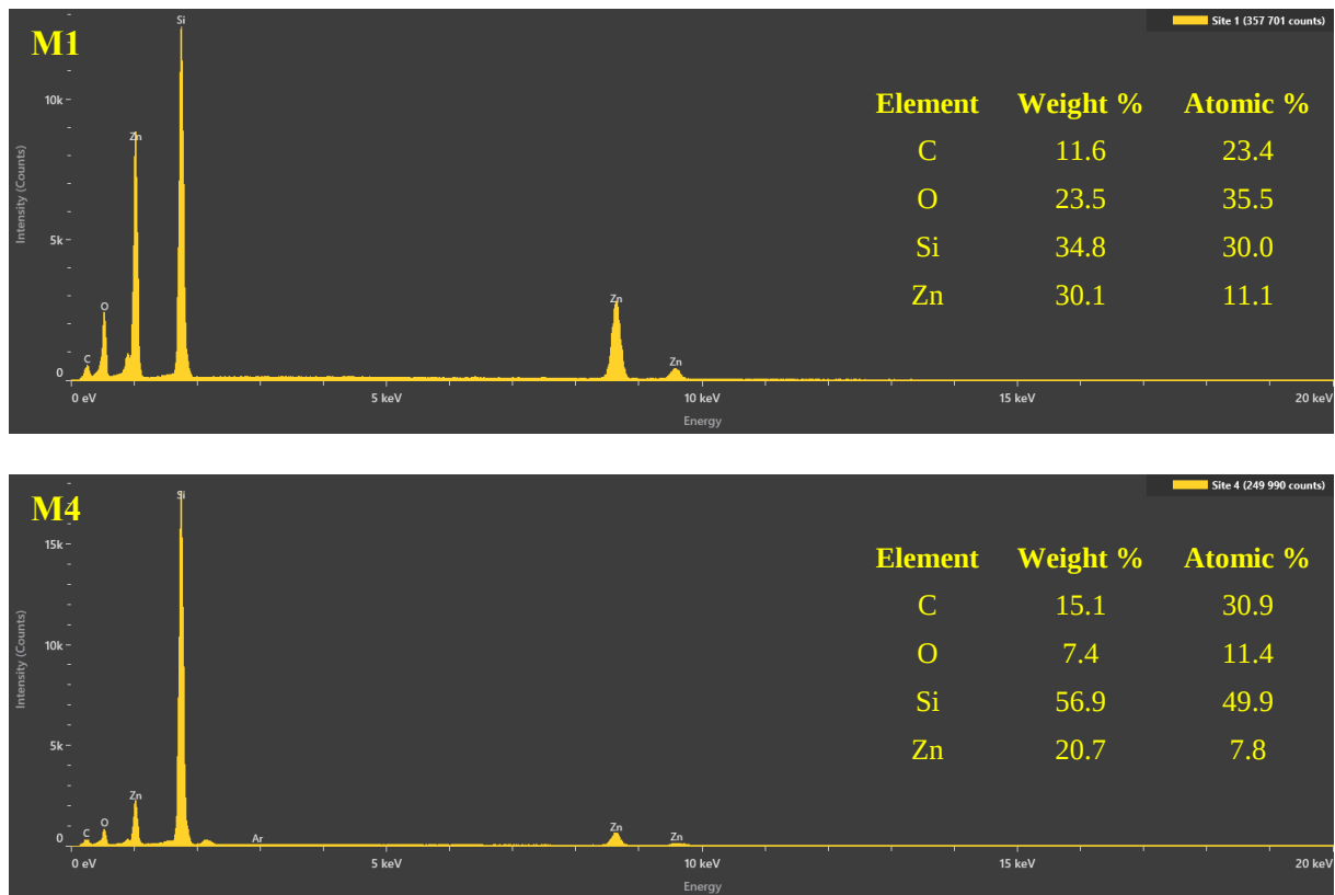
Figure 4: EDX spectra distribution and data of elements percentage for ZnO NPs deposited on a silicon substrate, synthesized by NTPJ for 15 min, using different methods to reduce oxygen percentage (M1 and M4).
